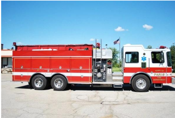
5512 a 1996 2000-gallon pumper tanker
